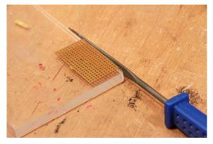
If there is no grinding wheel available use a fine file to clear up the edges, best in conjunction with a stable and crisp material underneath that gives guidance to the tool.
