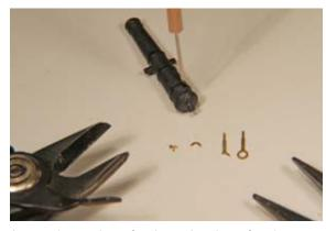
As an alternative of using wire rings for the breeching rings, the eyebolts can be used.
