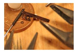
Take a wire of the needed diameter as core and bend another wire around it and cut the spiral into single rings. Open them sideways, stick them through the eyebolt and close it.
