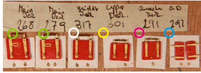
The different types of lids have different numbers of inside bolts, here shown lying underneath the lids. Lower and middle deck lids have two rings, upper and quarter deck have one ring on the inside.
