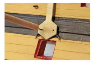
Spacers for the drilling of the holes for the lanyards. Hold spacer well, use a needle to mark the holes, remove the spacer and drill the holes accordingly.
