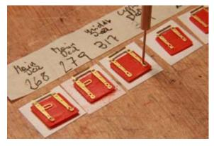
Use a needle to punch a hole for the ring bold through the hole in the fitting ...
