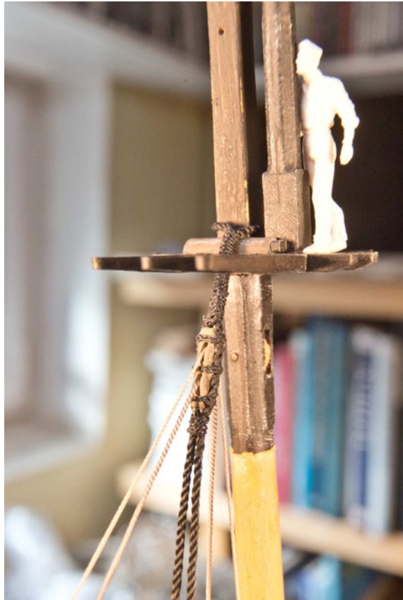
Sister blocks between the shrouds for the lifts and reef rackle pendants, clew garnets for the clew-lines and a long tackle for the foremast stay, which is hooked into the timber heads.
