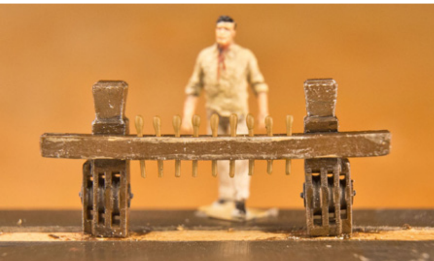
Front foremast bitt with 17 pins and additional rollers attached to the sides.
